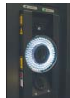
LED 8-segment oblique illuminators surrounding the objective lens
